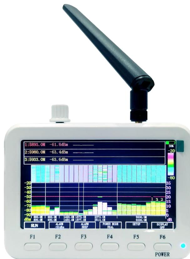
DOX (D03、D06) WIRELESS detector, built-in 21700 lithium battery ,is small and lightweight, through the micro USB interface 5V charger can be charged, detector with full charged can be used for about 7~8 hours. The operation frequency range is 10MHz~2700MHz and 30MHz~6GHz, and the statistics of the histogram of signal power in different frequency bands is displayed on the LCD. By configuring the frequency band parameters (the
